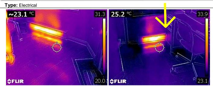
All electrical baseboard heaters were tested and were functioning well at the time of this home inspection. I recommend keeping furniture and textiles, like drapes, sofa away from the unit to avoid fire hazards and ensure your system runs efficiently.
